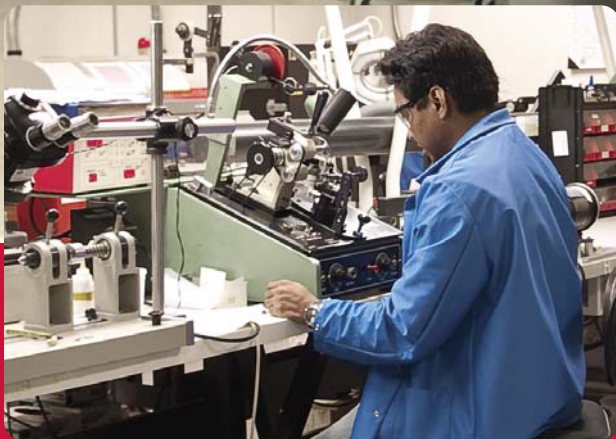
Left Precision winding equipment is used to insure compliance to customer specifications and tolerances. Above Microelectronics assembly lines dedicated to custom magnetics production.
